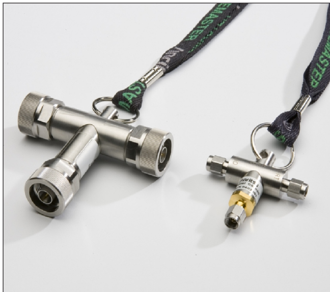
Figure 9. Convenient calibration artifacts (e.g., N and K) are available for the VNA Master Option 15, to provide the open, short and load standards for the calibration procedure.
