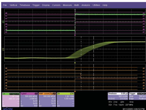
Figure 6. Sample-based pattern triggering generates 4 ns of trigger jitter (LeCroy WaveRunner with MSO option).
