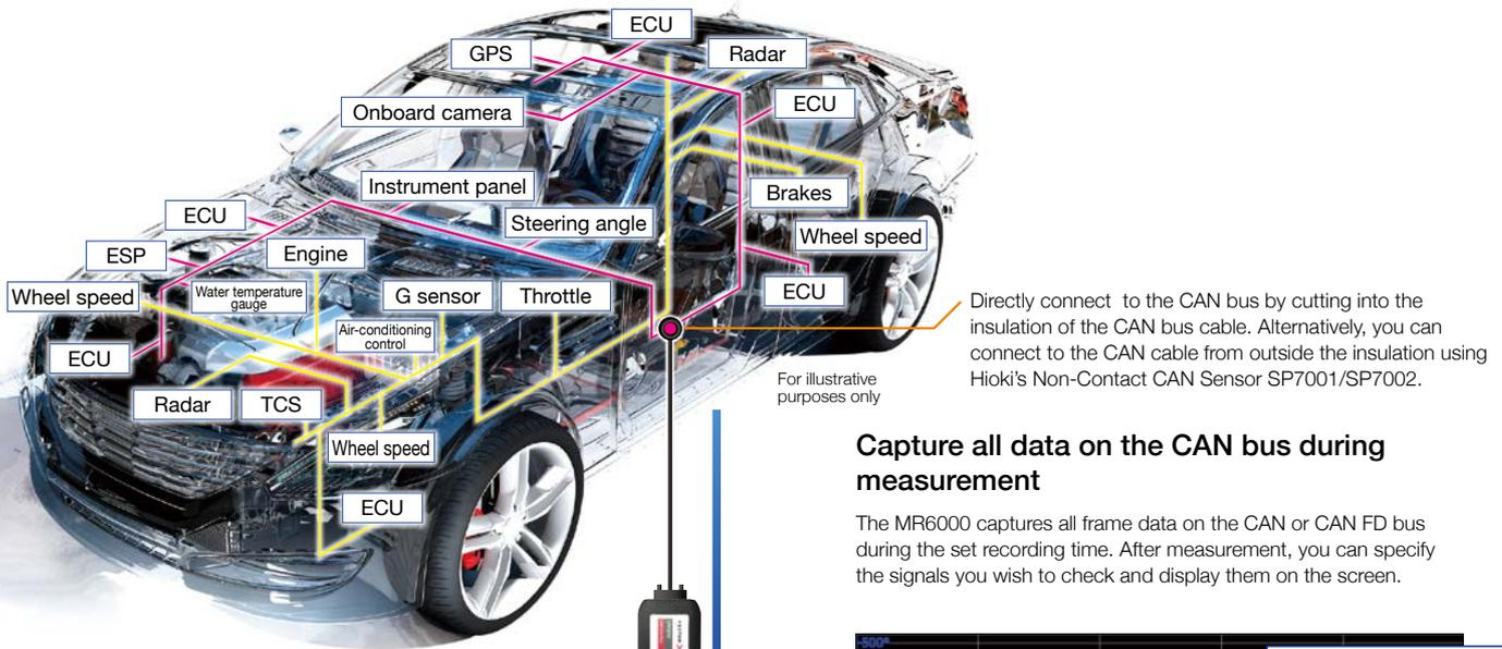
Directly connect to the CAN bus by cutting into the insulation of the CAN bus cable. Alternatively, you can connect to the CAN cable from outside the insulation using Hioki's Non-Contact CAN Sensor SP7001/SP7002.
