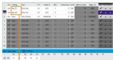
A shortcut key can be assigned to the transmit function.
