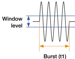
Calculate the time at which the burst signal is output
