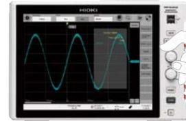
▲ Tap the screen and use the knob to move the trace cursor as desired.
