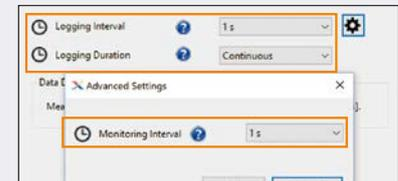
\*Monitoring interval ≤ Logging interval. The minimum interval depends on the network transmission speed.
