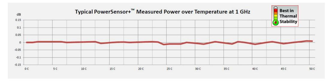
Thanks to our patented dynamic calibration system, LadyBug Sensors deliver full accuracy without user internal or external zeroing processes.
