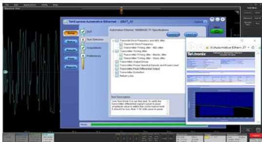
Automated compliance testing to the 1000BASE-T1 Automotive Ethernet standard
