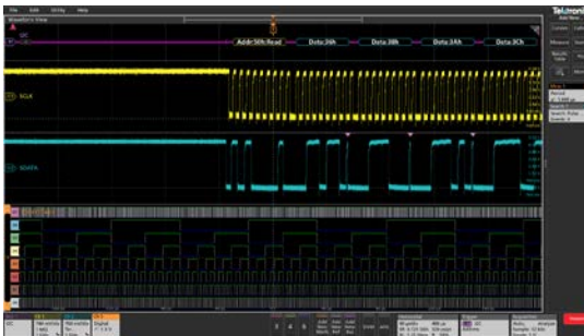
PC decoding synchronized with digital waveforms from a TLA058 logic probe
