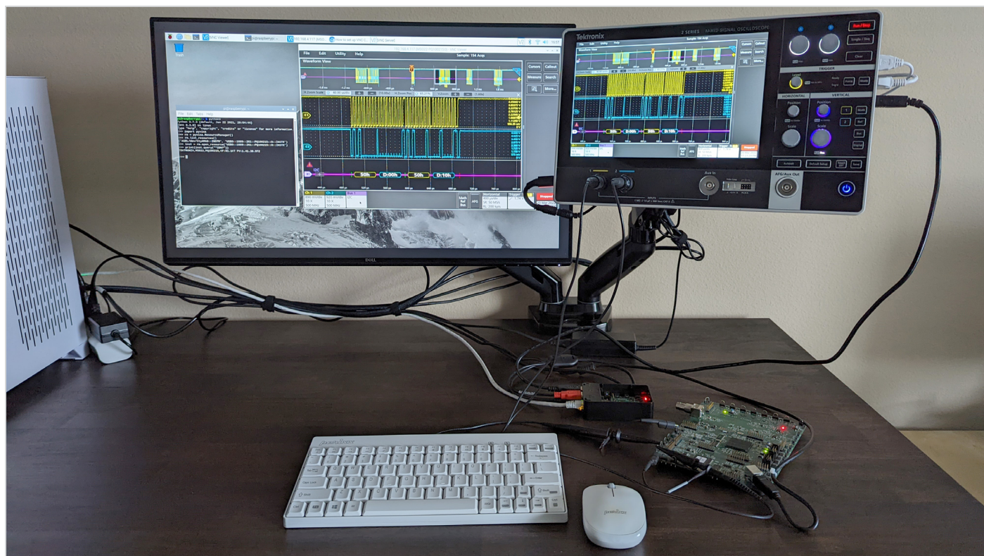
Figure 1: A quick setup for the Tektronix 2 Series MSO Mixed Signal Oscilloscope and a Raspberry Pi.
