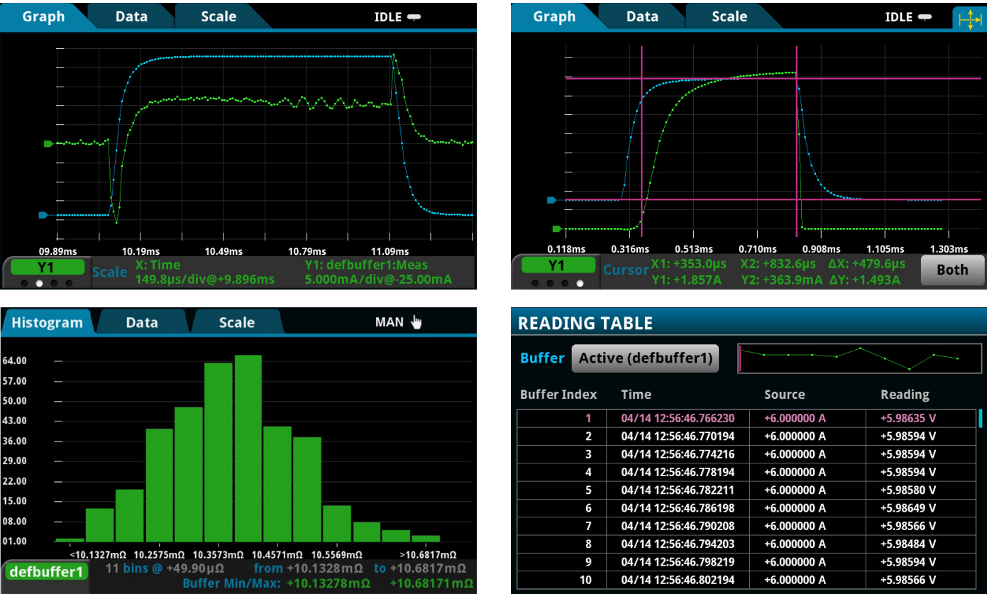
Figure 11: Built-in data display, charting, and spreadsheet export functions simplify converting test results into useful information.
