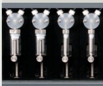
Syringe pump selection optimizes liquid volume range.
