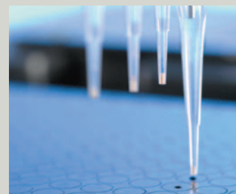
Protein digestion and MALDI target spotting with Zip Tips®
