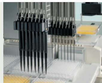
Combination of fixed and disposable tips on two liquid handling arms
