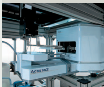
Robotic manipulator with extended Z-axis for access beneath worktable
