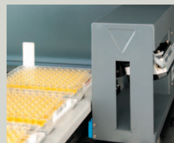
The PosID™ allows barcode identification of tubes and plates
