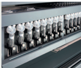
Syringe pumps optimize for each liquid channel
