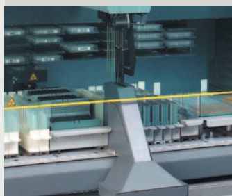
Low disposable tip ejection contains aerosol transmission
