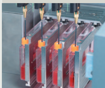
Tecan's Cellerity™ fully automated cell culture system pierces Corning® RoboFlask® septa
