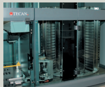
Individual random access with the high-speed carousel
