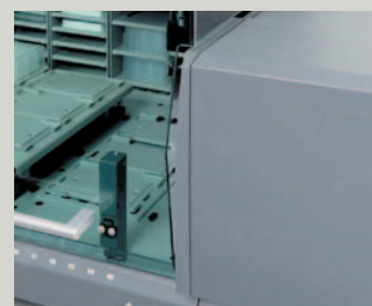
Personnel are protected by interlocked shields
