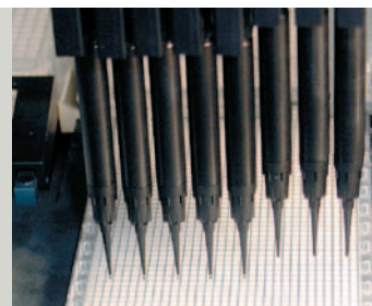
10 µl disposable tips pipetting into standard 1536-well plate
