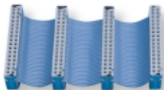
Figure 1. RTSI Bus Cable
