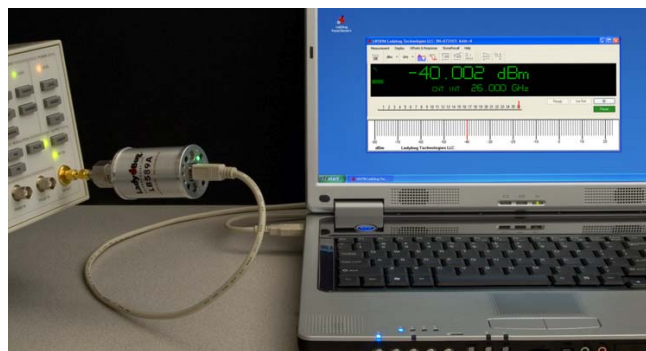
Test Setup for One Sensor Measurements
