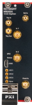
Figure 2. M9203A front panel with analog inputs and multiple I/O signals
