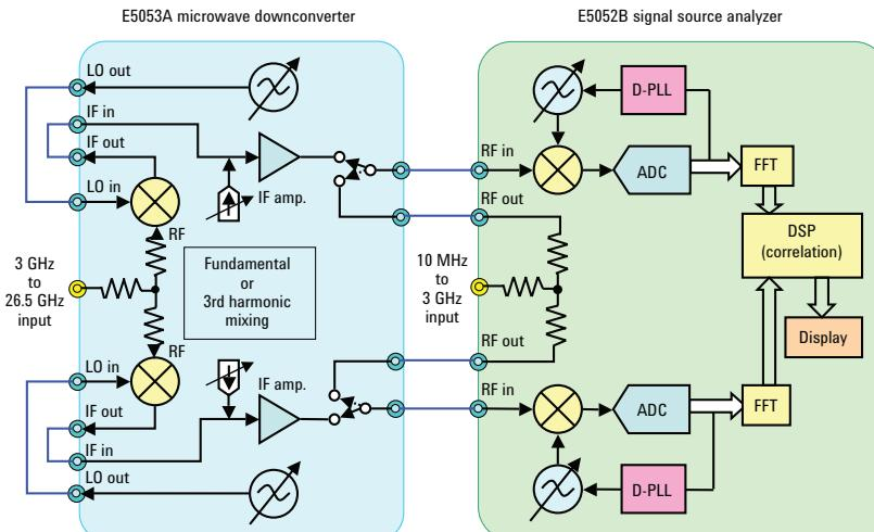
**Figure 10-1. E5053A with E5052B simplified block diagram**
