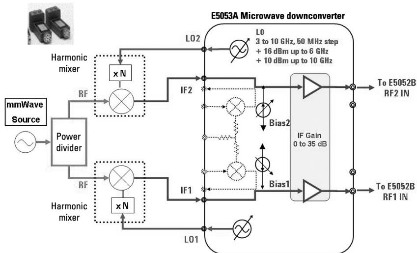
Figure 10-4. System set-up for harmonic mixers (E5053A + E5052B)
