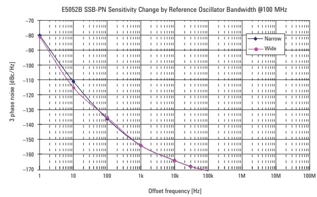
**Figure 1-5. SSB phase noise sensitivity change by reference oscillator bandwidth (SPD)**
