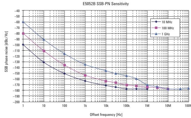
**Figure 1-1. SSB phase noise sensitivity (E5052B, SPD)**
