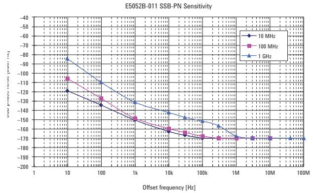
**Figure 1-2. SSB phase noise sensitivity (E5052B Option 011, SPD)**
