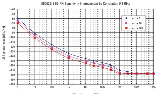
**Figure 1-3. SSB phase noise sensitivity improvement by correlation (E5052B, SPD)**
