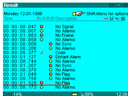
Fig 5 Log of errors and alarms with high-resolution time stamps
