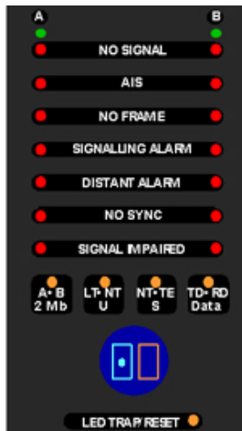
Fig 4 Line status LEDs. Detailed information on errors and alarms is shown in the display
