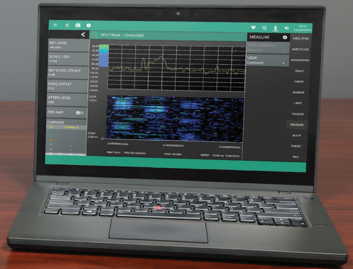
Laptop PC Running Remote GUI Application with Wi-Fi Connection to MS2085A/89A
