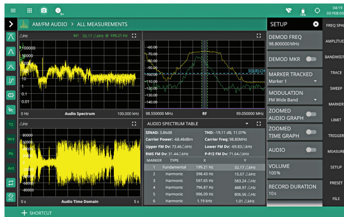
The AM/FM Modulation Measurements Screen Provides a Unique Simultaneous Display of Results and RF and Audio Spectrum
