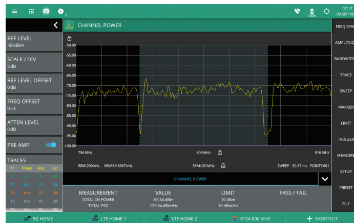
Measuring the Channel Power of an LTE Carrier between Adjacent Carriers
