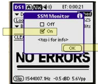
8..The SSM is displayed in Binary/HEX at bottom of screen, but may also be viewed as text by tapping msg. When viewing text, switch to Binary/HEX by tapping hex.
