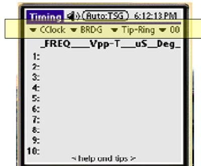
3..Tap the icon at top of screen: Auto:TSG and the test set will automatically begin sequencing through each of the ten inputs.
