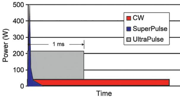
**Fig 1.** AcuBlade operating modes. AcuBlade is scanner software that allows beam to sweep given surface with extreme rapidity or to travel as straight or curved incision.
