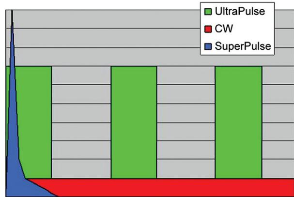
**Fig 2.** Laser output SuperPulse has higher peak power than UltraPulse, but clearly less energy (because blue area is smaller than green one). Amount of pulse energy determines tissue impact, provided both pulses are within thermal relaxation time of approximately 1 ms. CW — continuous wave.
