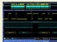
I 2 C serial bus decode showing address and data packet content.
