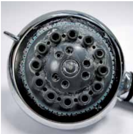
Symbolic picture showing a blocked dispense head
