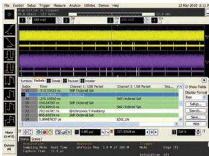
Isolate signal integrity problems from logic-level coding errors on bidirectional serial data streams.
