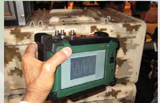
Universal standalone analysis and maintenance equipment (digital multimeter, oscilloscope, RF testing...)
